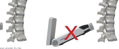
Tip: Arrange the scanning plane angle to be perpendicular to the spinal anatomy.
