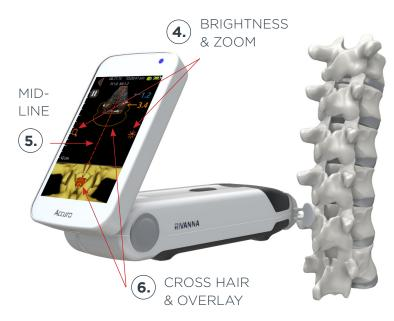
SCAN IN TRANSVERSE ORIENTATION, holding **Accuro** perpendicular to imaging surface. Red dashed line and cross hair indicate interlaminar space identified.
