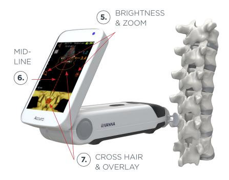
SCAN IN TRANSVERSE ORIENTATION, holding **Accuro** perpendicular to the spinal anatomy. Red dashed line and cross hair indicate interlaminar space identified.
