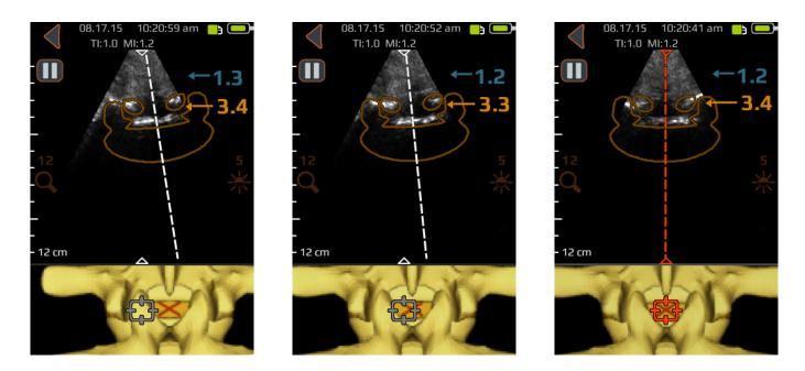
Move the device left or right to ensure the mid-line indicator is centered on the imaging screen (indicated by a dashed red line as shown).
